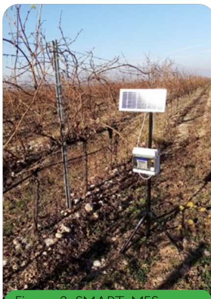
Figure 2: SMART-MES station for purpose of precision agriculture (vineyard) SMART-MES stanica za potrebe precizne poljoprivrede (u oblasti vinogradstva)
