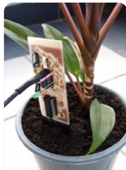
Figure 3: SMART-MES station for purpose of precision micro farming, left station, right, developed capacitive sensor.
